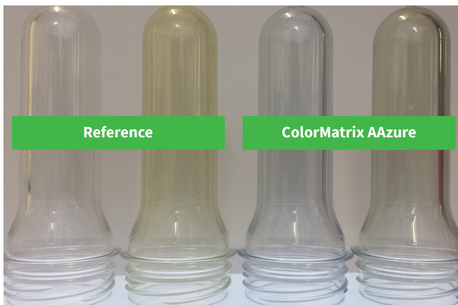
Impact of 5 Melt Heat Histories on Preform Color
